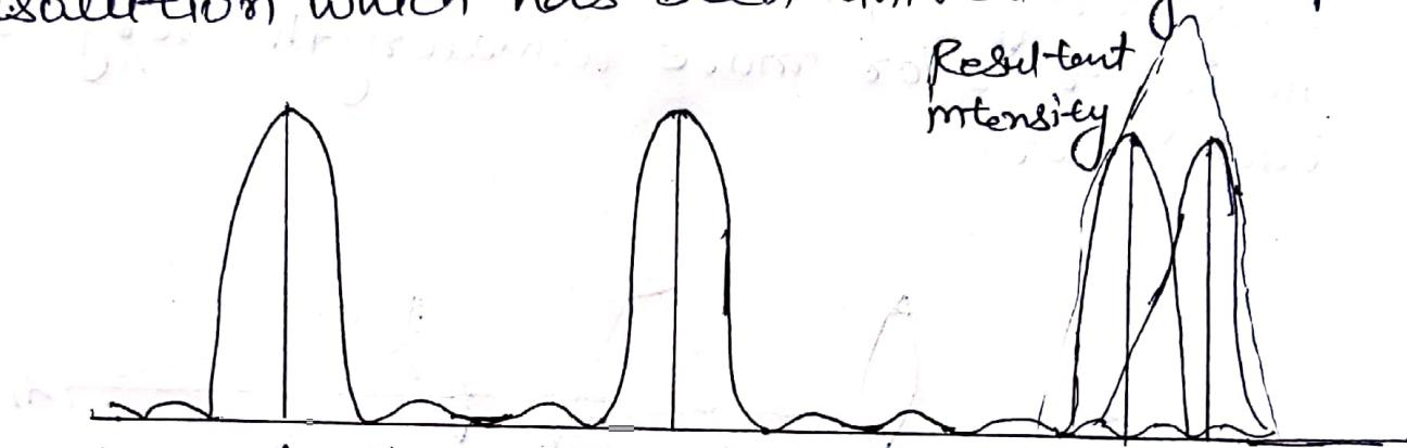
Two spectral lines of equal intensity are just resolved by an optical instrument when the principal maximum of the diffraction pattern due to one falls on the first minimum of the diffraction pattern of the other.
